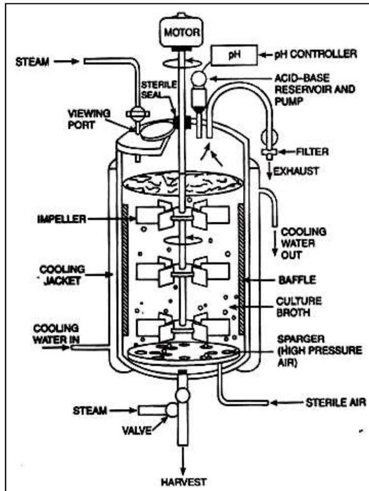
Fig.: An Industrial aerobic bioreactor (Internal View).
