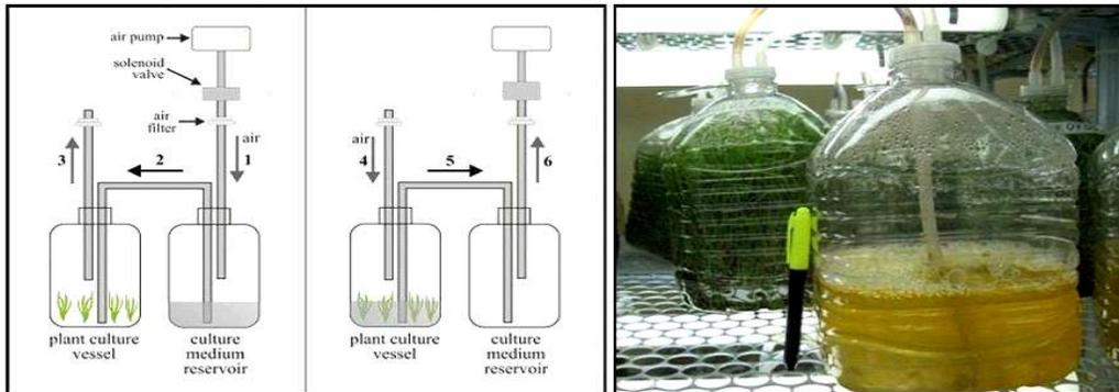
**Fig.: Temporary immersion bioreactor (TIB): The transfer of the medium to the plant culture vessel occurs by a positive pressure of the air pump and the explants are temporarily immersed, after this, the air pump starts and the medium returns to the culture medium reservoir (A) scheme, (B) picture.**
